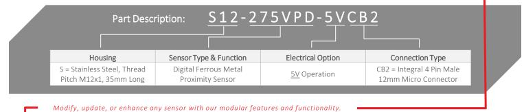
HOUSING - Aluminum, stainless steel, plastic, threaded, flange mount, customer specific
