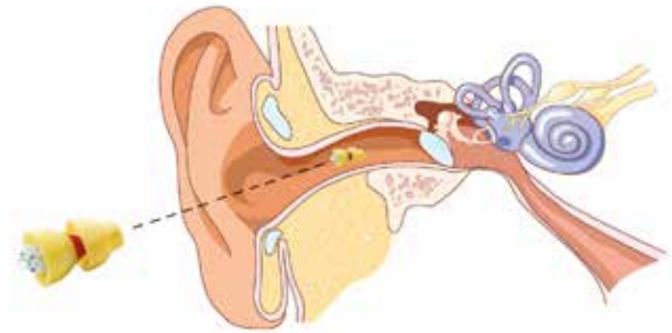
Figure 2. Completely In-the-canal hearing aid with integrated micro reed sensor.
