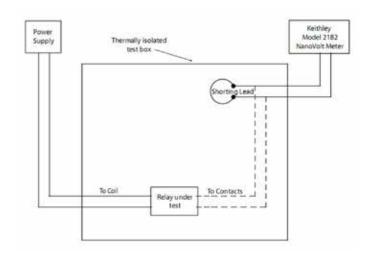
Figure 9. Single pole relay thermal offset voltage measurement setup.
