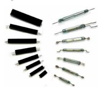
Reed switches from Standex-Meder are also robust enough to endure the conditions inside a vehicle. The switching element in their reed switch sensors is hermetically sealed, protecting the sensor from its surroundings. As a result, reed sensors can operate over a wide range of temperatures (-55°C to 155°C) and function in dirty, corrosive under-the-hood environments without any negative effects on their operating characteristics.
