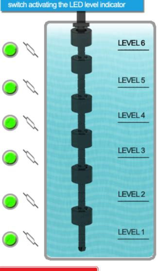
Magnets built into the floats move over the
