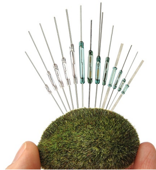
Reed Switches for a variety of Proximity & Fluid Level Sensing Applications
