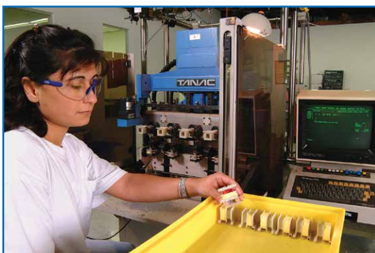
Computer controlled multiple piece winding up to 12,000 rpm.
