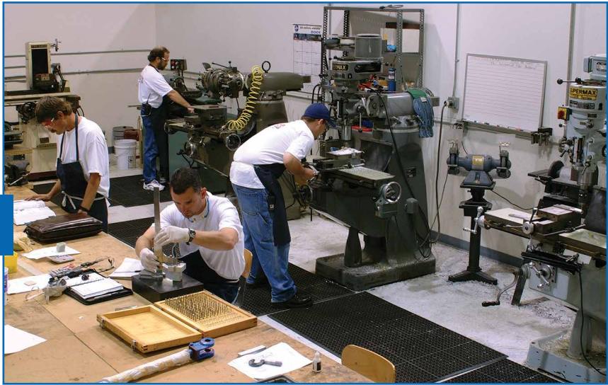
Complete in-house machine shop with core gapping capability.
