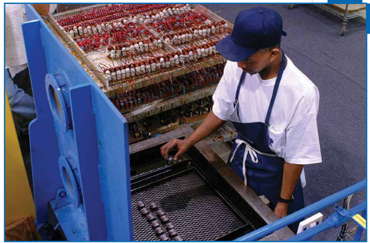
Vacuum varnishing with precise level control.
