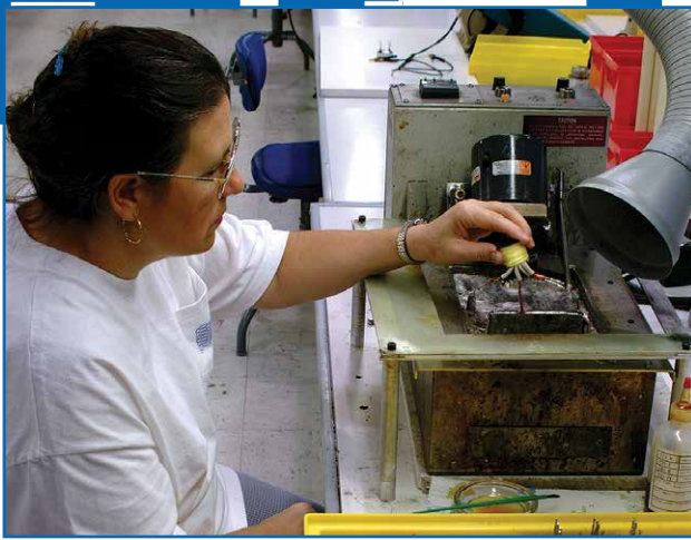
Wave soldering to eliminate contamination.
