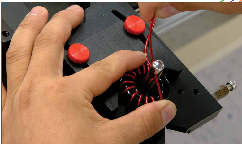
Heavy gauge toroid winding up to #8 AWG.
