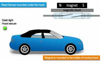
Figure 2. Reed Sensor is mounted inside engine compartment and magnet is mounted to the underside of the hood. A spring loaded ferromagnetic shunt is positioned between the sensor and magnet to shunt magnetic field.
