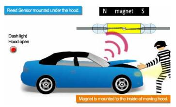
Figure 3. When the hood is opened the magnetic shunt springs out of position causing the magnetic field to actuated the sensor and signal the onboard computer to alarm.
