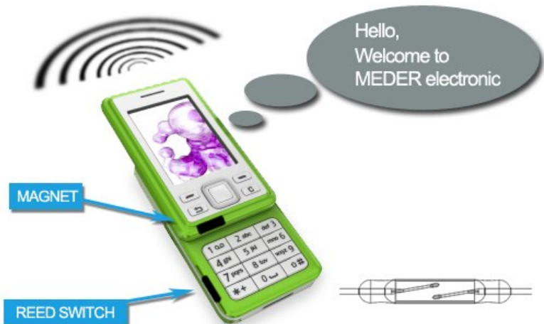
Figure 3. Phone open, Reed Switch is deactivated with magnet distance from switch.
