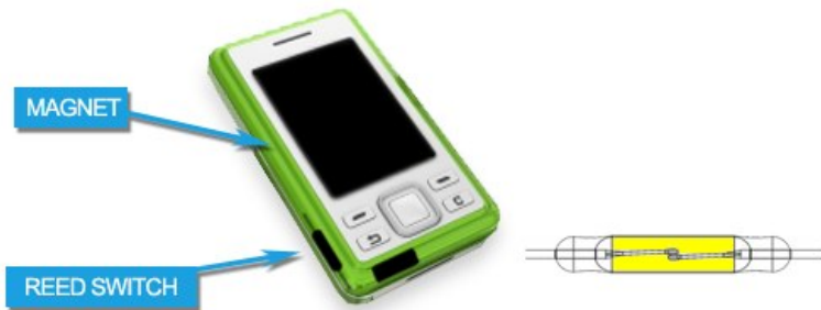
Figure 2.. Phone closed, Reed Switch activated while in proximity to magnet
