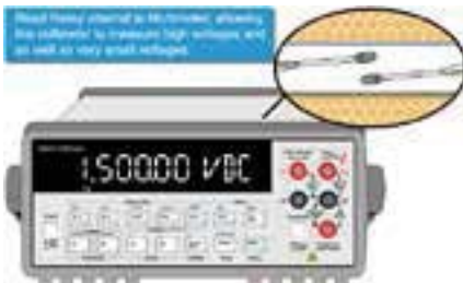
High End Multimeters Use Reed Relays to Measure Low & High Voltages
